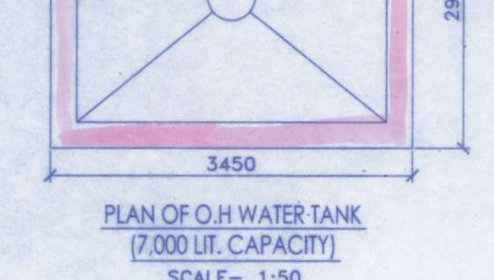
PLAN OF O.H. WATER TANK (7,000 LIT. CAPACITY) SCALE- 1:50
